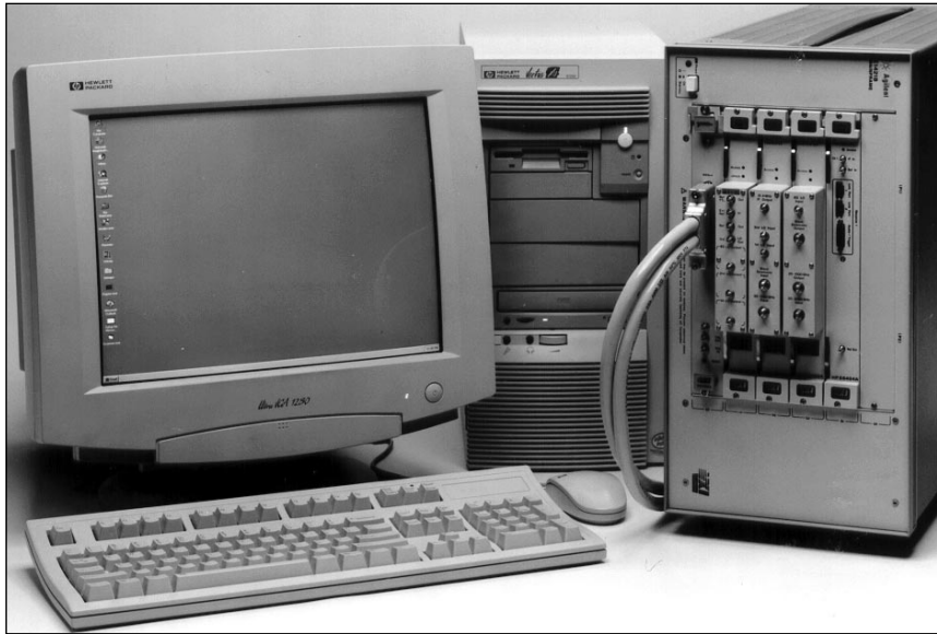
Agilent E6501A Option 003 receiver in optional six slot VXI mainframe with customer-supplied MXI interface, PC, and monitor
