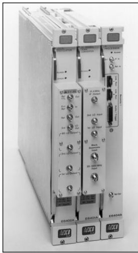
Figure 3. The E6501A receiver covers the 2 MHz to 1 GHz frequency range.
