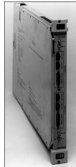
Figure 12. The E6404A dual channel IF processor VXI module (shown with Options 031 and 040) includes two Sharc link digital output connectors and one multi-pin analog audio output connector per mezzanine. The standard model includes only one mezzanine.
